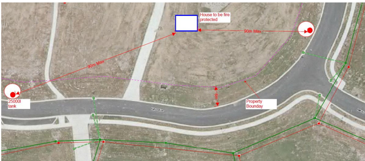
Figure 3 -Distance requirement and tank location
